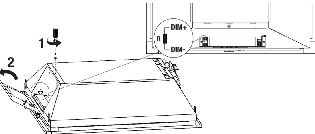
1) 0-10V dimming ranges from 10% to 100%.
