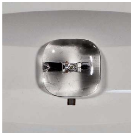
Largaluce lens (SY) installed at a height of 3 m illuminates a surface area of 11.3 × 11.3 m at 0.5 lux (128 m 2 )
