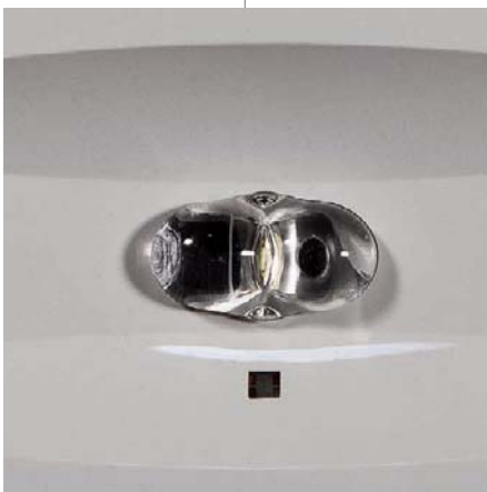
Lungaluce lens (ASY) installed at a height of 3 m covers an escape route of 17.1 m with 1 lux along the centre line and > 0.5 within 1 m
