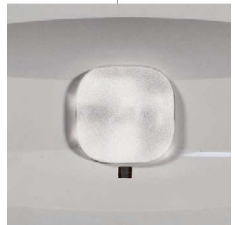
Diffusaluca lens (SY Opal) A wall mounted diffusa luce lens at a height of 2.5 m illuminates a surface area of 7 × 3 m at 0.5 lux (21 m 2 )
