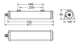
Acciaio Extreme surface wall mounting, surface ceiling mounting, chain or wire suspension emergency luminaire
