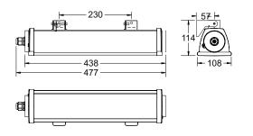
Acciaio Extreme surface wall mounting, surface ceiling mounting, with swivel bracket emergency luminaire
