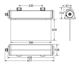
Acciaio Exreme surface wall mounting, surface ceiling mounting, with swivel bracket exit sign luminaire
