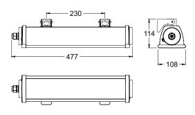
Acciaio surface wall mounting, surface ceiling mounting, chain or wire suspension emergency luminaire
