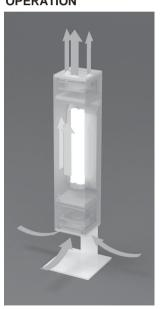
The sanitization unit consists of an axial fan intake system that draws air inside the closed chamber containing the UV-C source, where the sanitization process takes place. The UVoxy® replaceable cartridge is installed inside of the module. Replacement is quick and ensures the sanitization characteristics of the appliance are maintained over time. Use an original UVoxy® Beghelli spare part (code 26720).
