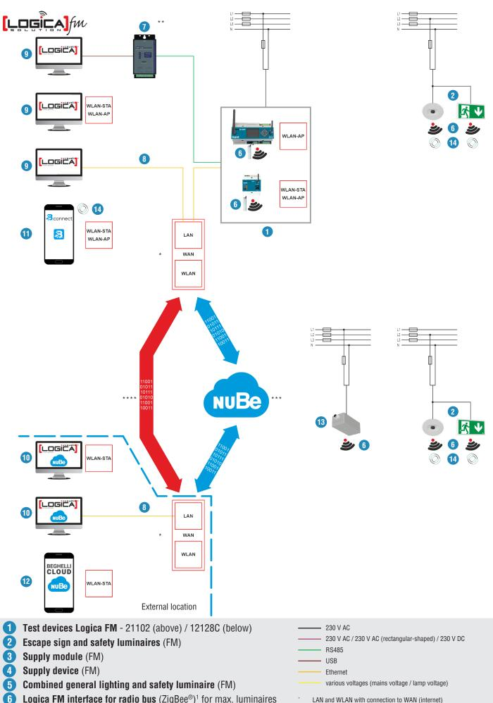
6 Logica FM interface for radio bus (ZigBee®)<sup>1</sup> for max. luminaires / supply modules / supply devices:
