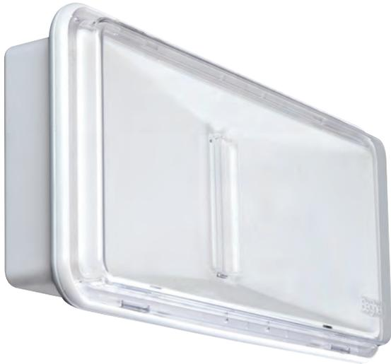
A luminaire equipped with an innovative lens that increases the lighting performance making it possible to increase the centre distance between luminaires and the pictogram lighting uniformity. The optical design offers special anti-glare and excellent light diffusion characteristics thanks to a clear methacrylate diffuser that hides the LED source while maximising the luminous flux. LiFe batteries for extreme ambient temperatures (**quality guaranteed for 5 years**).
