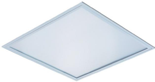
Lyra LED is a luminaire for mounting in ceiling module M600, M625 and plaster ceilings. Its body is made of steel sheet finished by powder technology varnishing, colour white RAL 9003, with diffuser with microprismatic optics. The degree of protection is IP20. It fits perfectly in computer labs, large and small offices and lecture halls.
